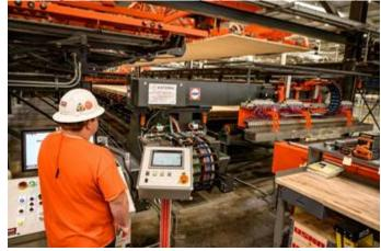
Press operator Ricky Miller uses a layup press to glue and layer long and short boards together at Katerra, a cross-laminated timber factory that opened Friday in Spokane Valley. Katerra says the 270,000 square foot CLT facility is the largest in North America. (Colin Mulvany / The Spokesman-Review)
